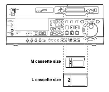
Align the center of the cassette with the center of the insertion slot, and press it in gently.
